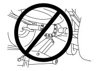
8. Remove the lug nuts with the lug wrench.
